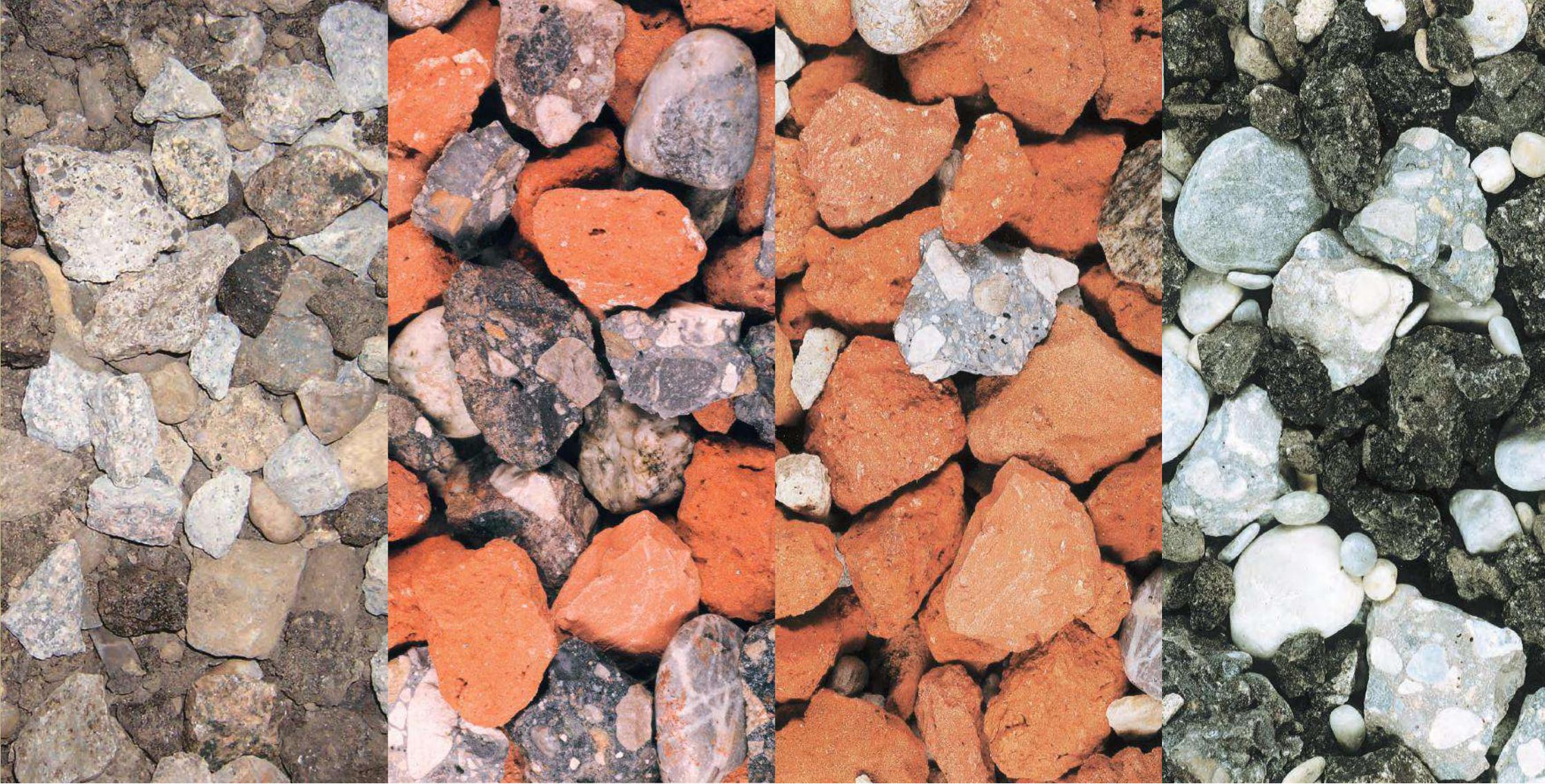
**RG** – Recycled granulate from natural and/or recycled stone with a content of at least 50% concrete and/or asphalt
