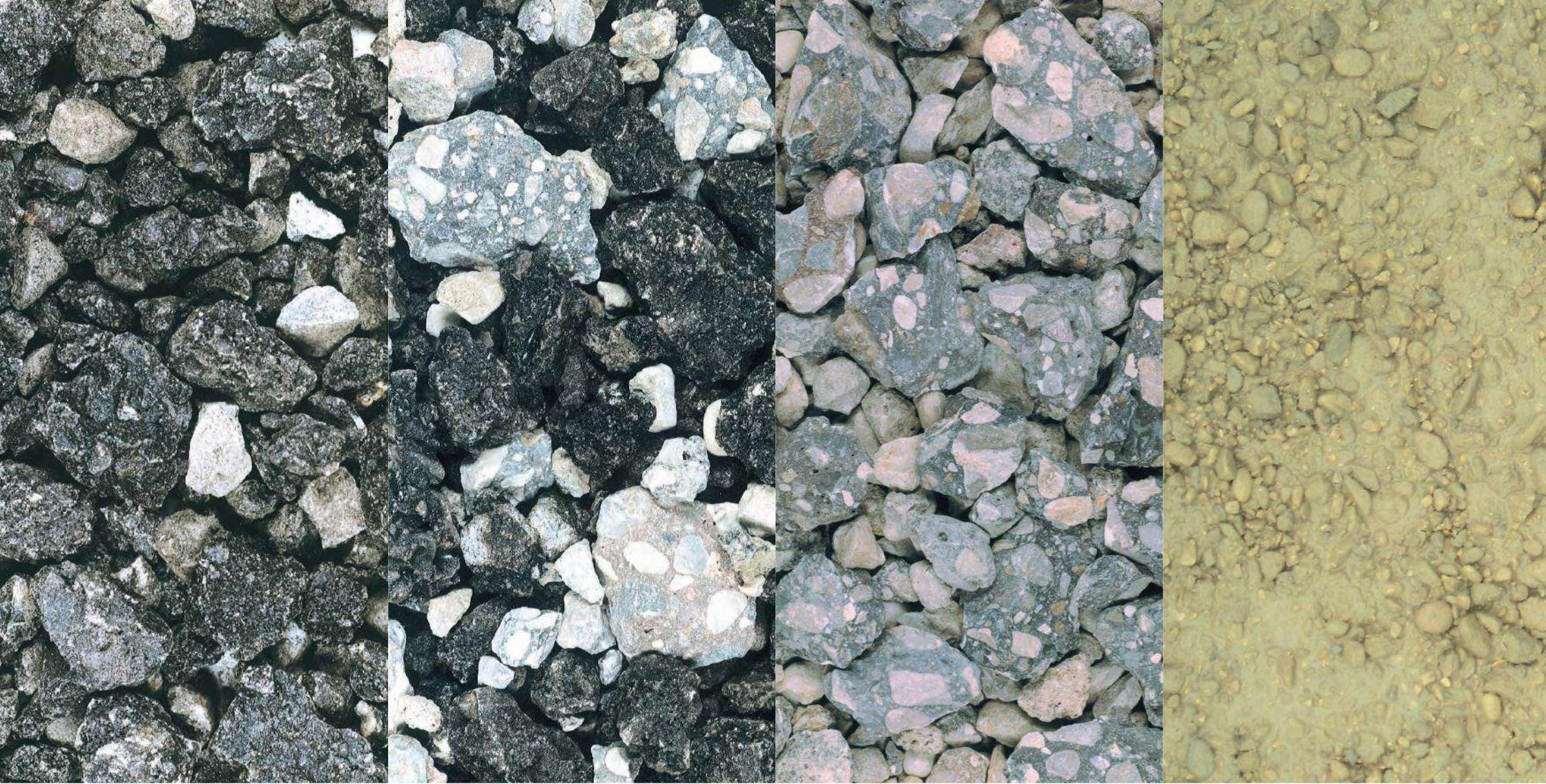
**RA – Recycled crushed asphalt granulate (mainly asphalt)**
