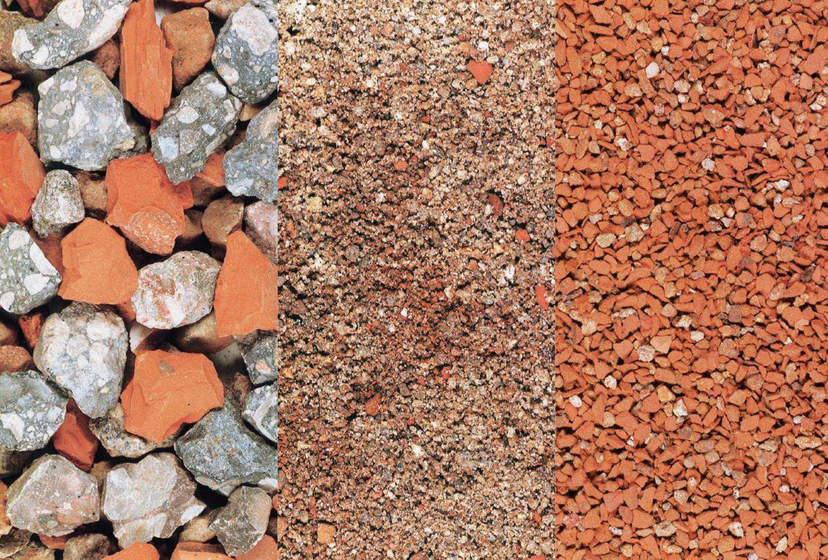
**RMH – Mineral residual building material (concrete, brick, natural stone)**
